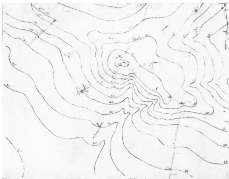
CROSS-ROADS AND CONTOURS REVISED ON PLANE-TABLE: DETAIL TO BE FITTED FROM AIR PHOTOGRAPHS
